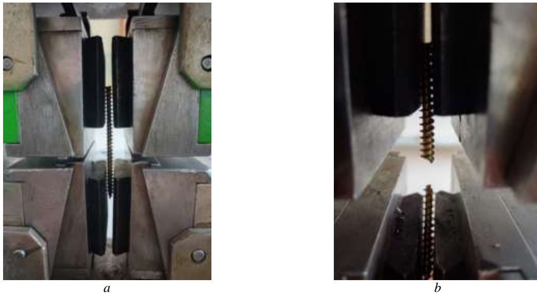
Fig. 5 Failure of a steel self-tapping screw: a – appearance before failure; b – appearance after failure. Photo by Ihor Bakan
