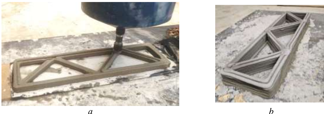
Fig. 1 View of the beam structure: a - during the printing process; b - after completion of the printing process. Photo by K. Sirenok
