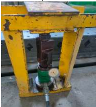
Fig. 5 Calibrating the hydraulic jack and pressure gauge.
