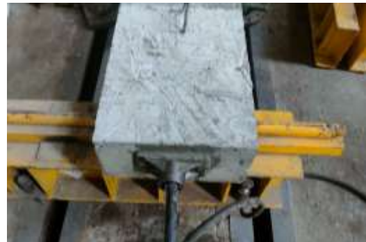
Fig. 7 Fragment of a beam of the second series with installed anchors. Photo by: Vynokur V.
