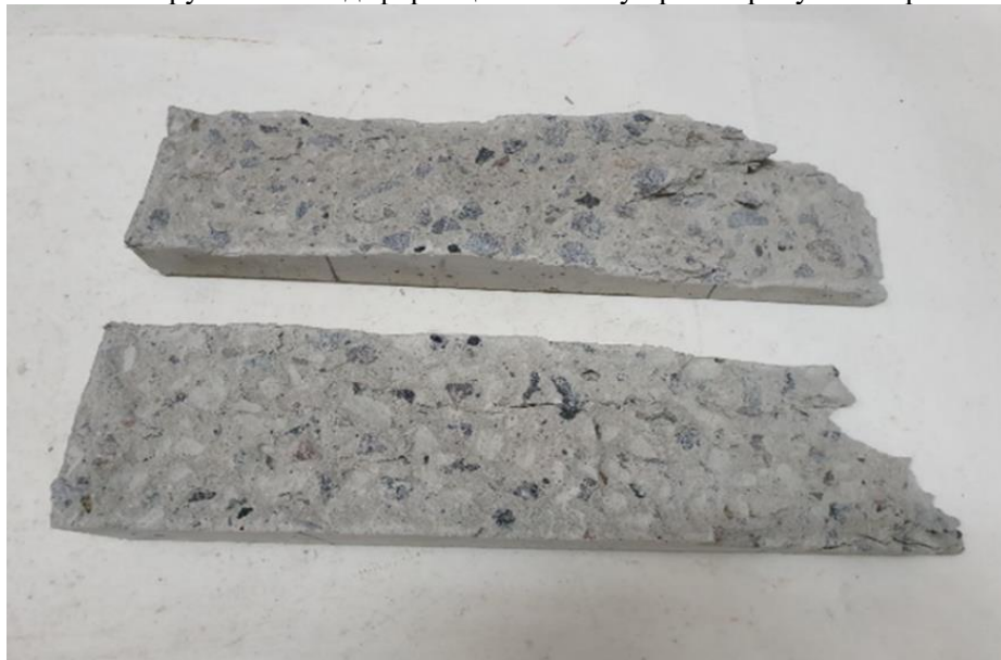
Fig 3. Structure of the internal surface of concrete prism P-3 14 (Photo by D. Zhuk)
