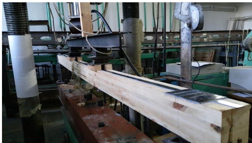
Fig. 4 The curing process of the adhesive when bonding the composite strip reinforcement Sika CarboDur S-512 to the timber beam. Photo by Gomon, 2022
