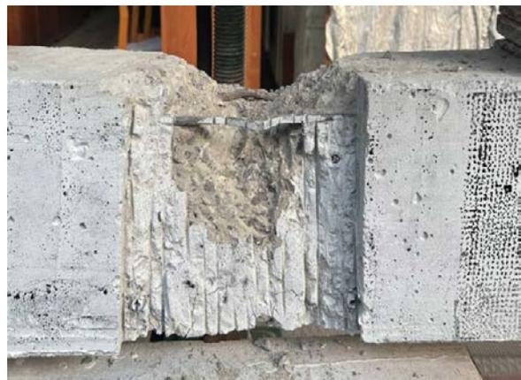
**Fig. 9.** View of the reinforced concrete beam after the experiment from the damaged side.
