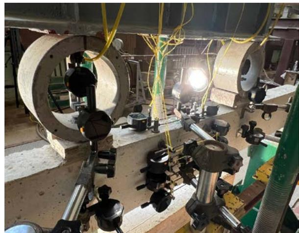
**Fig. 3.** Placement of the micro-indicators.
