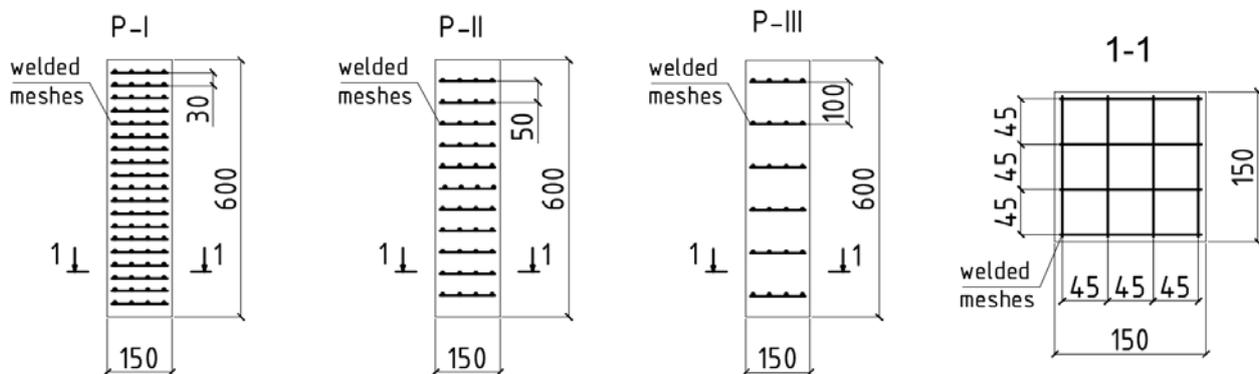
**Fig. 2.** The designs of the experimental samples
