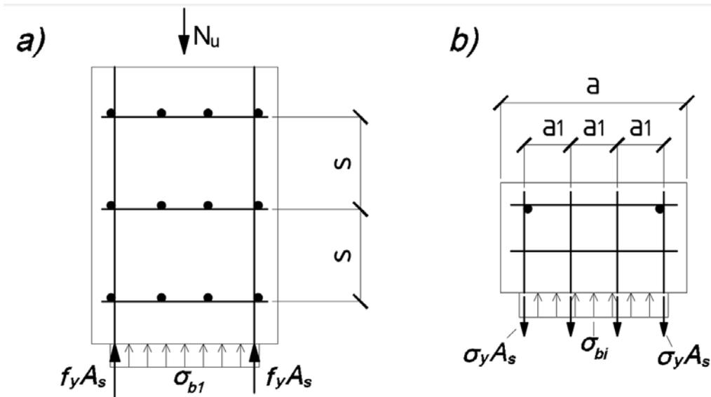
**Fig. 1.** Calculation model of a reinforced concrete element with transverse mesh reinforcement at the stage of ultimate equilibrium: a - external and internal forces in a flat horizontal section; b - external and internal forces in a flat vertical section
